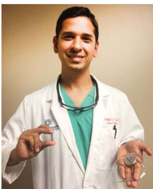
Dr. Karthik V. Prasad, compares a traditional pacemaker (right) with the new Micra ® Transcatheter Pacing System (left). The Micra TPS is one-10th the size, attaches directly to the heart and requires no cardiac leads.
